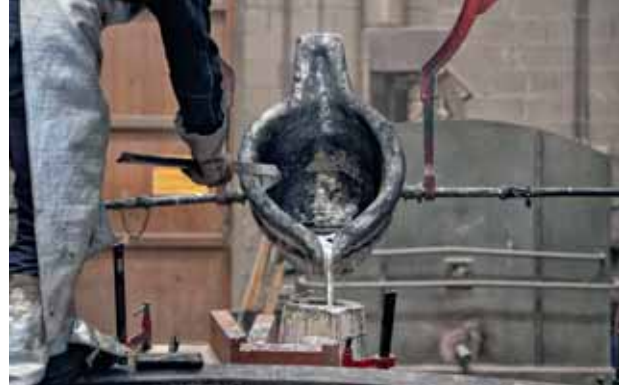
Casting the lead © Palace of Versailles, S. Giles
